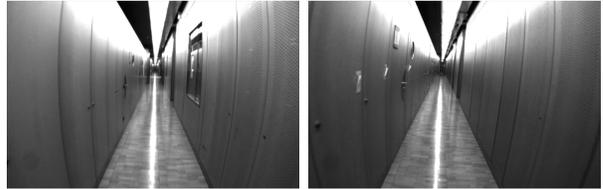
Fig. 4: A non-matching pair of frames from the CLA F dataset. Even though they look alike, the places are more than 20m apart. Using just keypoint descriptors leads to a localization failure due to the extreme visual aliasing. Visual context helps to disambiguate the locations – small cues let us reject false positive landmark matches.
