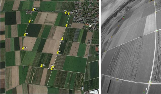
**Fig. 3:** **Left:** Landmark positions in UTM coordinates. **Right:** Hand-labeled feature positions (green) and reprojected landmark locations (red) given the camera pose estimated by the PNP.
