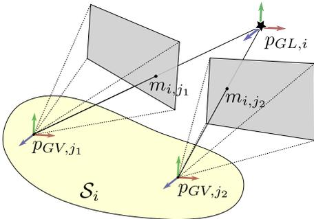
Fig. 3: A landmark located at  $p_{GL,i}$  is observed from a set  $\mathcal{S}_i$  of keyframes located at  $p_{GV,j}$ . For each keyframe, the location of the landmark in the image plane is given as  $m_{i,j}$ .
